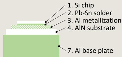
New base plate results in higher thermal conductivity between junction and case and an increased thermal-cycling performance
